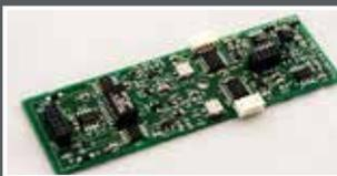
**ANALOG I/O MODULE:** Enables the Iridium to receive and transmit analog signals such as 4-20 mA, 0-20 mA, 0-10 VDC, etc. All signals are fully isolated.
