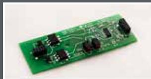
**ALARM OUTPUT MODULE:** Enables the alarms that are built-in to the Iridium to be transmitted externally via relay contacts.
